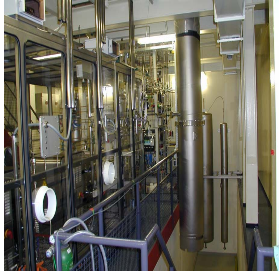
cryogenic distillation column with 2.7 m active length and 55 mm diameter.
