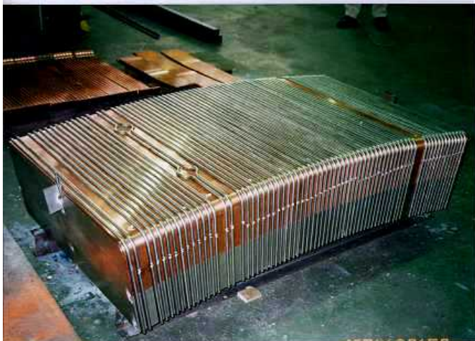
Assembly of steel tubes and DS Cu plates
