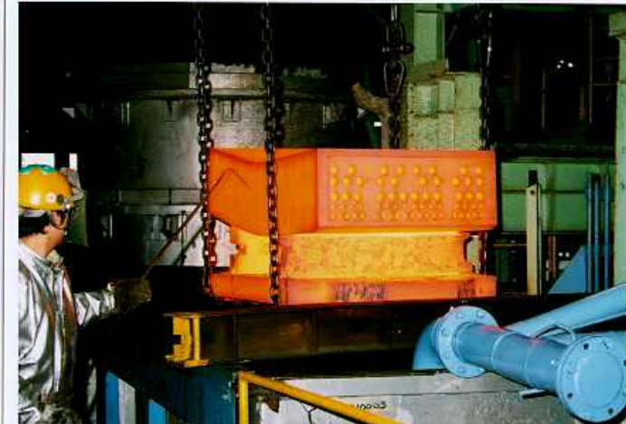
Steel block after solution heat treatment (1010-1054 °C)
