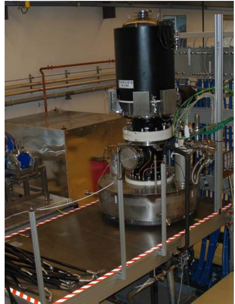
First prototype gyrotron installed in the SC magnet - ready for operation
