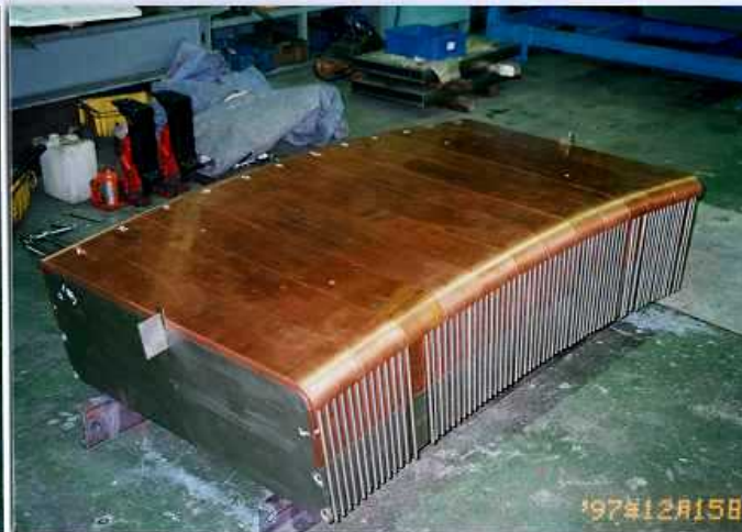
Final assembly of FW and shield block
